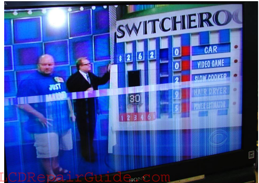
GATE DRIVER FAILURE
