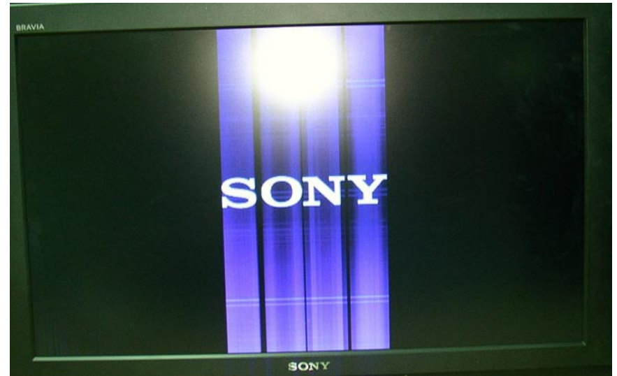
MULTIPLE SOURCE DRIVE IC FAILURE
