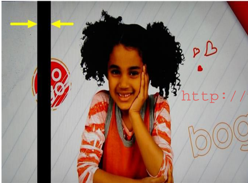
SOURCE DRIVE IC FAILURE
