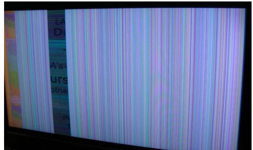
MULTI-COLORED LINES. NOTE THE PRESENCE OF SOME ACTIVE VIDEO INDICATING THE VIDEO PROCESSOR IS NOT THE CAUSE
